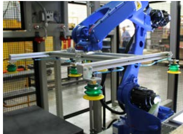
Sheet feed robot with precision vision guidance
