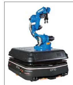
AGV enabled robot with vision guidance
