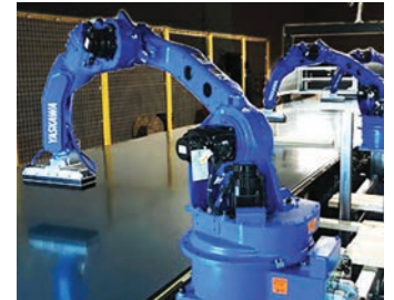
Pick and pack robot with vision guidance and conveyor tracking
