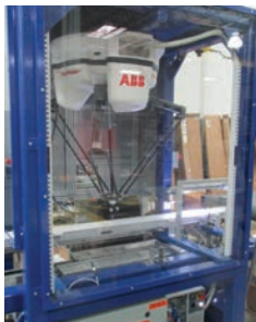
High speed pick and place robot for wash down applications
